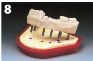
8 Remove model-former from base. Cross-shaped section glide in the sleeves which stay in the base. Bottom part of pins is readily accessible for pushing due to corresponding depth of model-former and length of pin.
