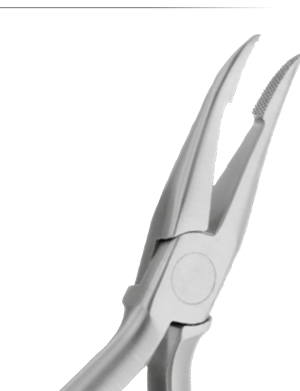
Ultra Slim Weingart Pliers 678-200 Ultra slim, 45 % slimmer at tip than 678-202, tapered 20° tips with serrations, useful for placement and removal of archwires.
