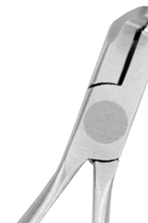
Universal Cut & Hold Distal End Cutter 678-101 Wire size: < = .012" to .021" x .025" (.30 mm - .53 mm x .64 mm) When used intraorally it safely holds the cut portion to be discarded. Patient comfort is enhanced by the smooth, tapered tip.
