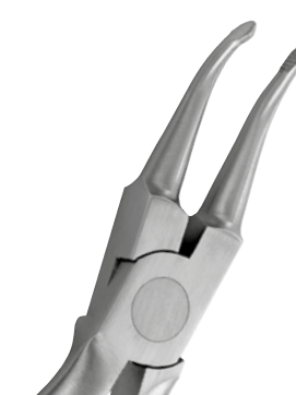
How Pliers, Offset 678-204 Wire size: < = .030" (.76 mm) Similar to the straight How pliers, except tips are angled at 40° for accessing lingual and other hard to reach areas.
